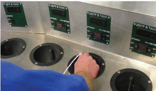
REOTEMP uses a combination of fixed point temperature calibration cells and fluid-filled calibration equipment to perform temperature calibrations from -321°F to 2,372°F (-196°C to 1,300°C). REOTEMP also offers pressure calibrations from inches of water up to 30,000 psi. Our friendly and knowledgeable calibration technicians will ensure your instruments have the accuracy required for your application.
