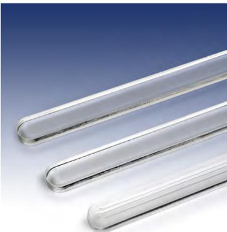
Replacement gauge glass, gaskets and mica shields. Borosilicate glass offers high visual clarity, greater chemical and thermal shock resistance, and high pressure safety. Gaskets and Mica Shields are also available.
