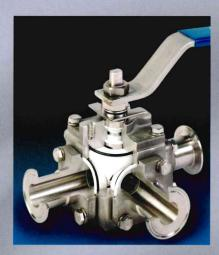
These PBM Multi-Port and other valves feature Direct Mount Actuation, which uses the valve stem as an integral part of the actuator drive to eliminate the side load and vertical load that can cause leakage.
