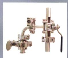
This permits sampling of steam for purity and safety isolates trap for ease of maintenance. While some assemblies require multiple valves, PBM's Steam Trap is a single valve that performs three functions, saving both space and cost. True-Bore® port design, standard on the steam trap valve, minimizes pockets and dead space in the through path, and prevents puddling where contamination could occur. Vertical or horizontal installation and various actuation packages are available.
