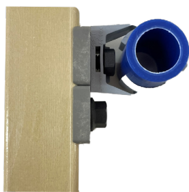
FRP Strut – Maximum Column Load at 60" Span = 1,047 lbs. with 3:1 Safety Factor
